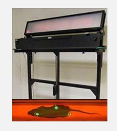
Cat Walk (motor) - Place animals on a pathway that captures the footprint placement in order to assess gait and locomotion
